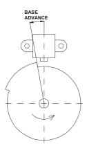
**Correction** - Correction of the advance of individual cylinders [°].
